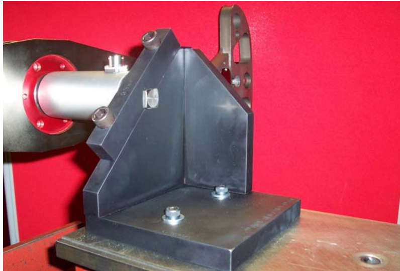
Figure 2. Transducer clamped in a mounting bench for an unsupported beam calibration. The fit of the squares and rigidity of the mounting plate are important factors
