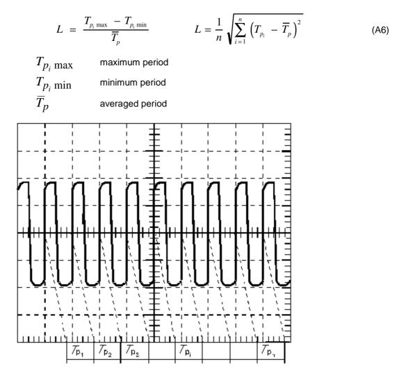
Fig. A7: Time base linearity check. Screen display in the completely balanced state at ideal linearity
