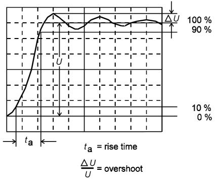
Fig. 7: Determination of the rise time
