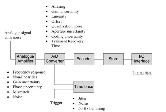
Fig. A6: Uncertainties of measurement in the digitizer, block diagram
