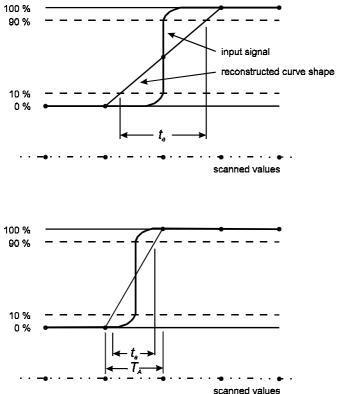
Fig. A2: Uncertainties of measurement of a step function
