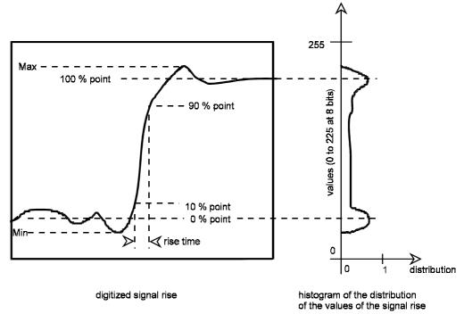
Fig. A3: Determination of the 0 % and 100 % points
